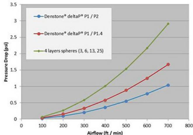
Figure 4: Denstone® deltaP® media pressure drop advantage vs. spherical support media. Source: Saint-Gobain NorPro
