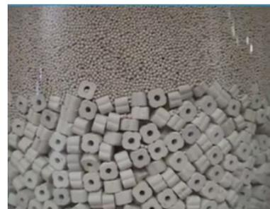
Figure 2. After 90 hours, testing shows Denstone® deltaP® retains catalyst particles with only minimal migration at the side wall. Source: Saint-Gobain NorPro
