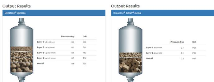
Figure 5. Results from the Pressure Drop Estimator show a significant decrease in pressure drop when utilizing Denstone® deltaP® vs. Denstone® spheres.
