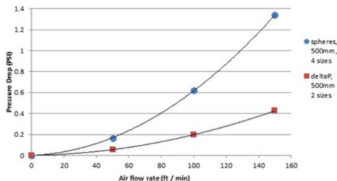
Figure 6. Pressure drop variation when air flow rate is adjusted and all other inputs remain constant.
