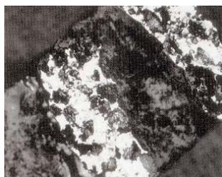
Enlarged example of MacroTrap® media with carbon particles.
