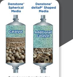
Typical support media loading configuration (not to scale).
